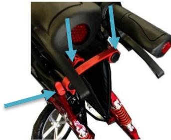
Push downwards on the seat rails to engage the locking mechanism.
