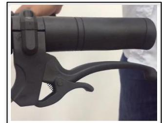
**Free parking brake: holding the brake lever and the small switch will release automatically; in the meantime, to release the parking brake for using rollator freely.**
