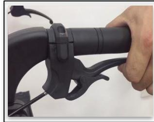
**Parking brake: using the finger to hold the small switch and pull the lever; it can be parked at the third position.**
