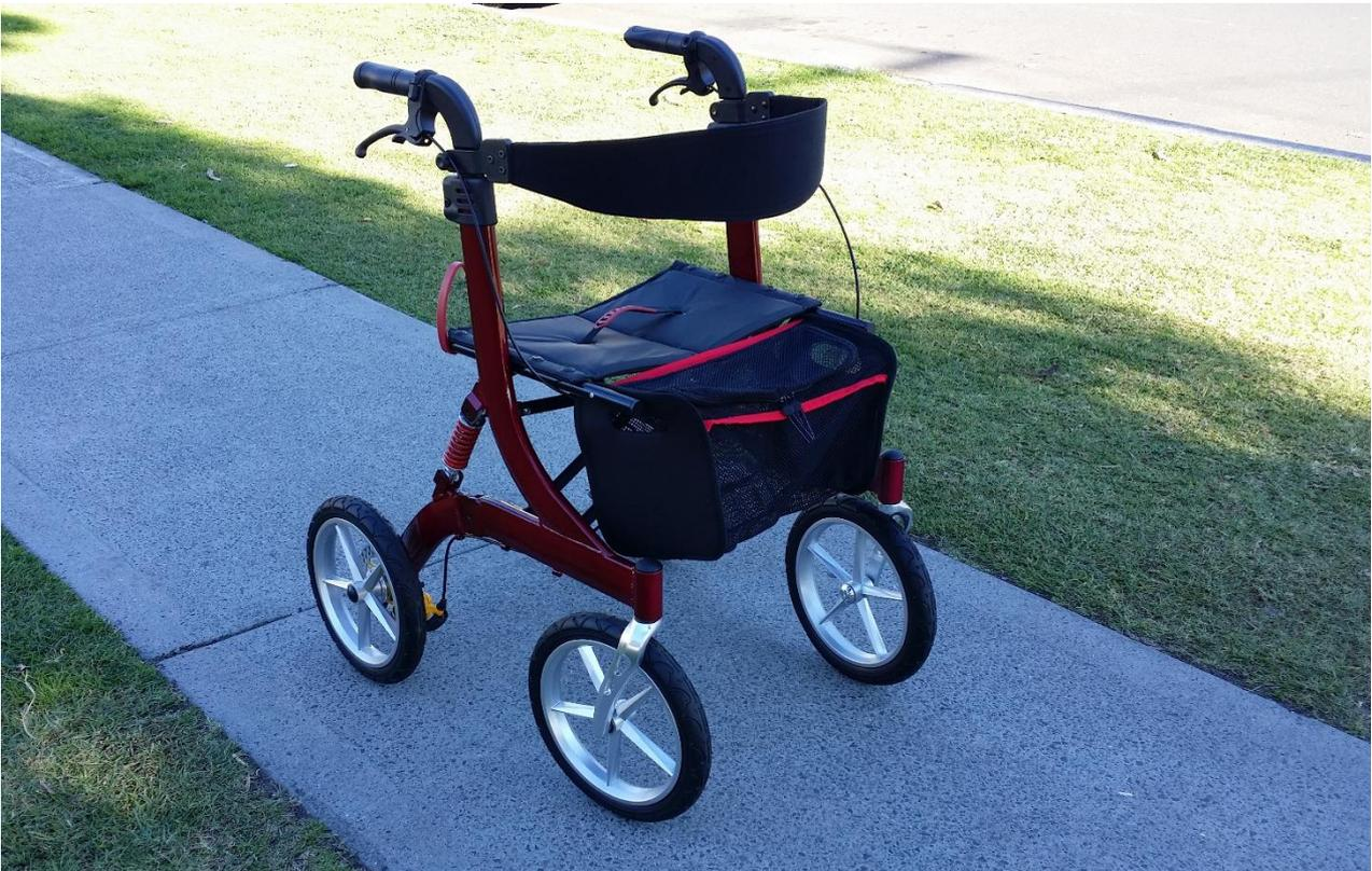
With Disc Brake and Suspension
